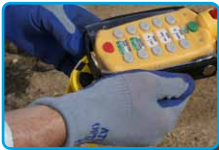
The operator can control the boom up/down, in/out and left/right with the wireless controls.
