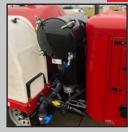
Protecting the positive displacement blower is a key part of extending the life of your Jet Vac. A cyclonic pre-filtration into a 3 micron washable reusable filter media, provides the protection you need when vac'ing wet or dry materials.
