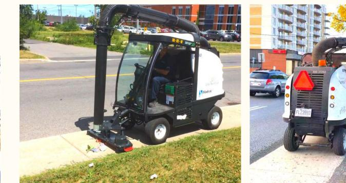
**Ergonomic 6-position robotic joystick allows** effortless displacement of the boom
