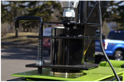
Stress-free boom rotates around hose
