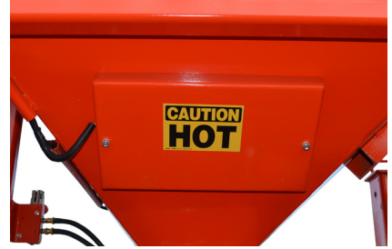
Hopper Heating System
