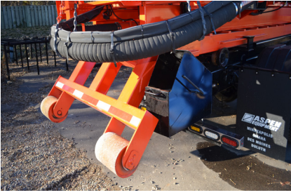
Rollers Allow Easy Loading And Unloading
